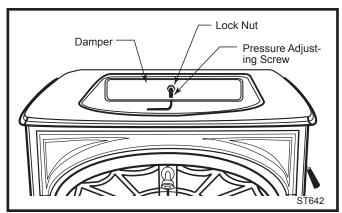
Fig. 31 Adjusting the damper.
